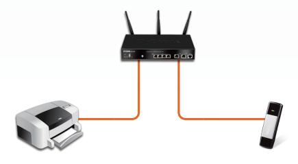
Supports one (DSR-150/250/500) or two (DSR-1000AC) USB 2.0 devices to extend functionality.
